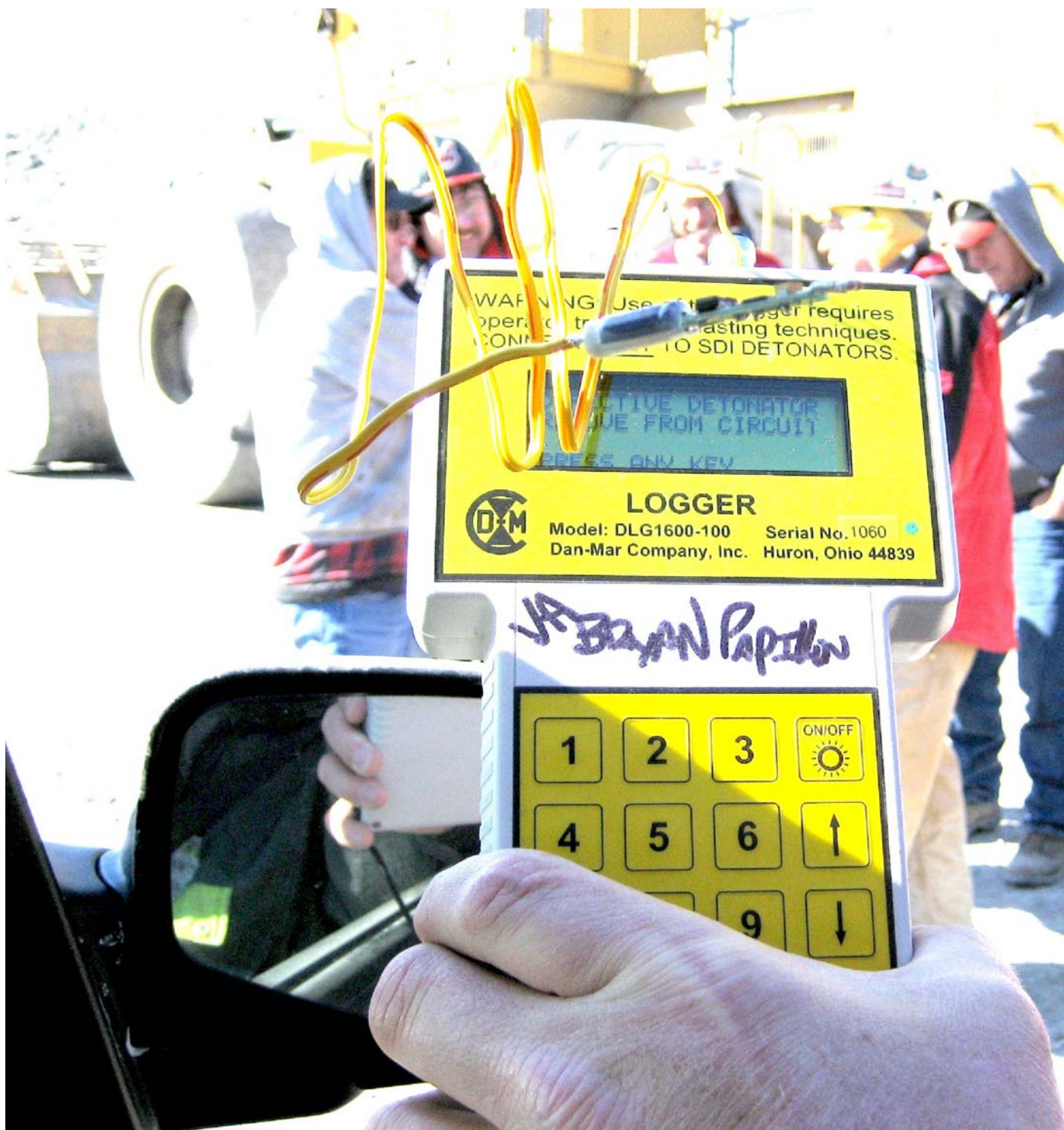
Figure 9 – Dash 100 Logger Showing Defective Detonator (Dummy)
