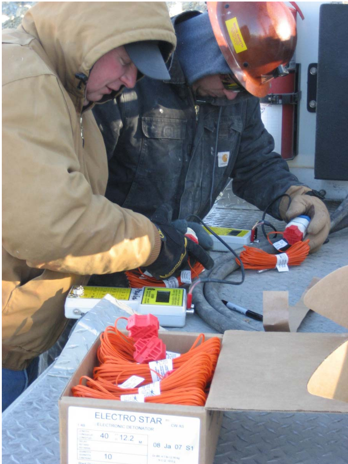
Figure 5 – Austin Electro*Star Electronic Detonators with Connector Block
